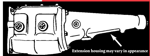
352 TREMEC 9 bolt top cover; first gear synchronized
